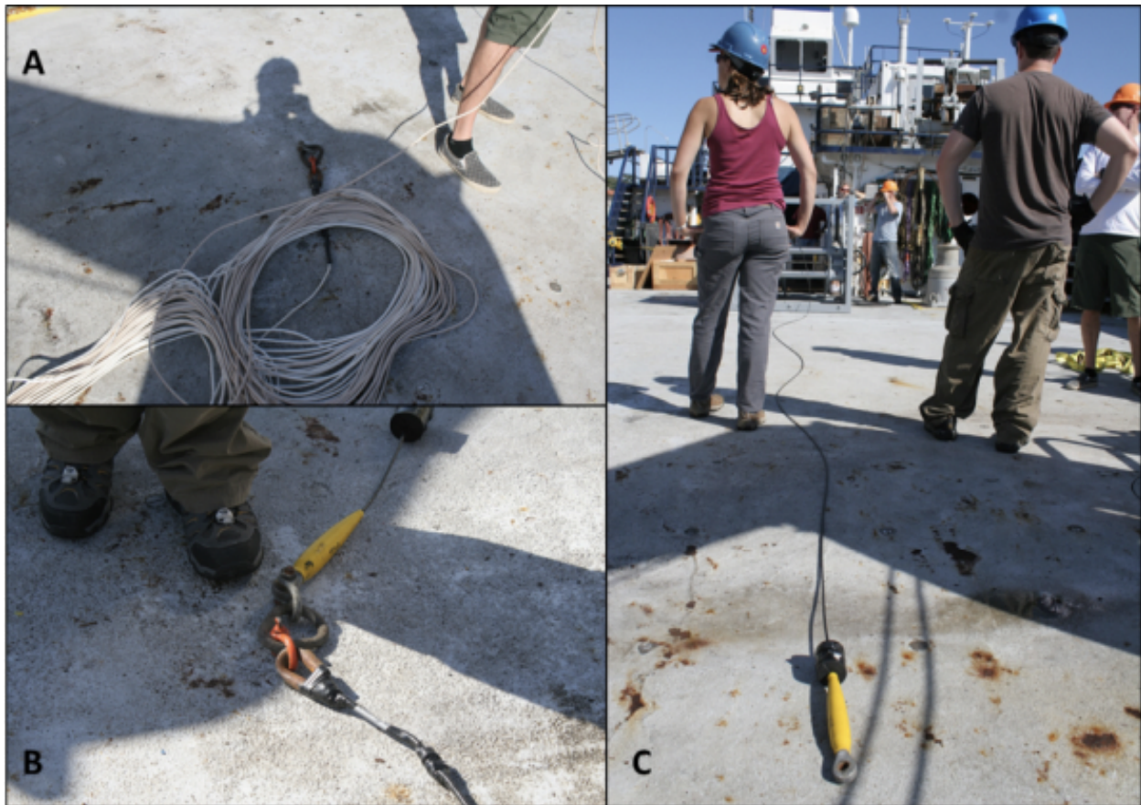
Figure 10: Deployment setup - (A) Backing line to be attached to the winch terminated with thimble; (B) Connection of rope line to the top of the Wirewalker coated wire connected with a D-Ring and shackle; (C) Rope line and most of Wirewalker coated wire spooled.
