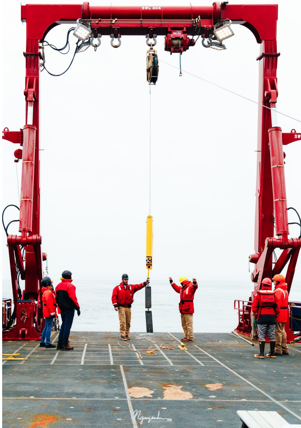
Figure 14: Final moments of a Wirewalker being retrieved. Photo Credit: San Nguyen aboard the R/V Sikuliaq.
