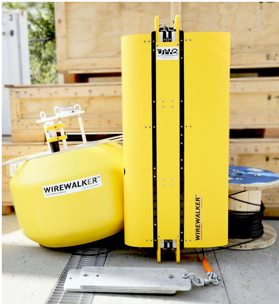
Figure 1: The Wirewalker Profiling System consists of a surface float, profiler, profiling wire, and downweight.
