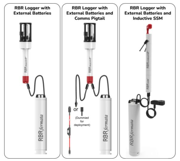
All scenarios where an end cap connector is present can connect the logger (MCBH-6-MP) to a battery canister (eg RBRfermata, MCBH-6-FS). A 12V power supply is typical, but other outputs may be present if the WW includes additional sensors (such as an ADCP). While the Gen3 RBR loggers handle a wide range of voltages (refer to RBR manual), the SSM is limited to 12V.
